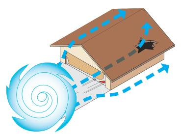
If you live in high wind and cyclonic areas, it's necessary to engineer your garage door a little differently to ensure it withstands the particular stresses it may be subject to and minimise the potential damage to your home.
