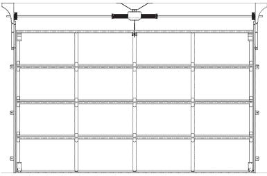
Max door height: 3.5m, Max door weight: 110kg, Max door area: 12m<sup>2</sup>
