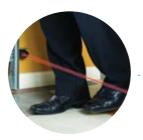
The Photo Electric Beam is designed to detect an obstruction while the door is closing and to send a signal to the opener to reverse or stop the door movement. It helps to protect your family from injury and your car from the damage caused by contact.
