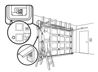
**One Button Close:** Opener can be closed by pressing only the ENTER button if the one button close feature has been activated. This feature has been activated at the factory. To activate or deactivate this feature press and hold buttons 1 and 9 for 10 seconds. The keypad will flash twice when the one button close is active. The keypad will flash four times when one button close is deactivated.
