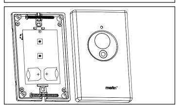
NOTE: The wireless wall button supplied with your opener should be preprogrammed by the factory. If adding a new wireless wall button, program into the opener before mounting the unit.
