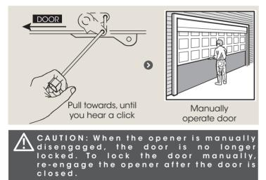
WARNING! When operating the manual release (while the door is open) the door may fall rapidly due to weak or broken springs, or due to being improperly balanced.
