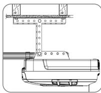
**Ceiling Beams that run parallel to the door requires:** 2 x perforated L shape metal strips and
