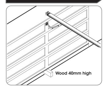
WARNING! If the door fails these tests, put the opener into manual mode, only operate the door by hand and call for service.
