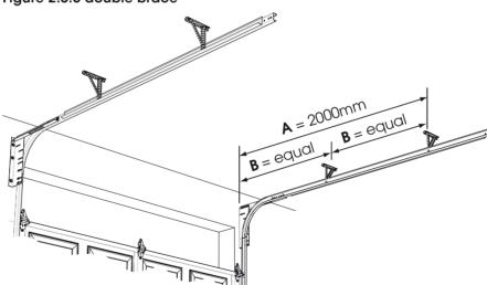
Figure 2.5.4 installing the safety stop
