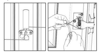
Figure 3.1.5 bending lock strike
