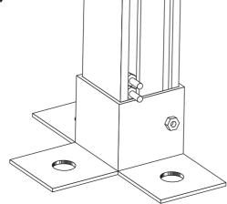
Assemble the "U" bolt as shown and fit over the top of the aluminium brace Figure 2.7.5.
