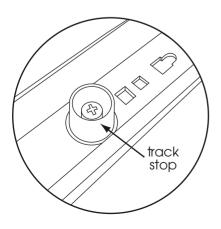
Safety stops must always be fitted at the end of each horizontal track.
