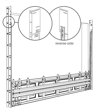
Now make sure the track aligns with the previous vertical marks and secure the top of the track to the structure using the specified fixings on the DTCM drawings.
