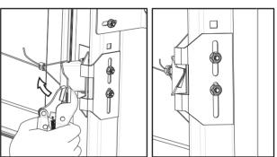
Figure 3.1.6 modification to lock when tracklocks are fitted (not supplied)
