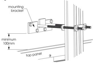
Slide the heads of 8 x  $\frac{1}{4}$ " hex head bolts 4 into each side of the aluminium brace, ensure they are in the slots shown in Figure 2.11.4. Loosely fit  $\frac{1}{4}$ " nuts to the 8 bolts this will become a spacer.
