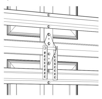
Now stand the aluminium brace in position, ensure it is plumb in line with the hinges, adjust the 'U' bolt so that it fits comfortably in the lintel bracket and the brace has 5-8mm clearance from the panel reinforcing, Figure 2.11.2.
