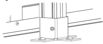
Stand the brace in position make sure it is hooked in place at the lintel and insert three dome head (S) fixing screws into the three floor anchors.
