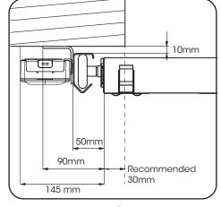
PANELIFT® (PFT) with optional Auto-lock measurements for vertical track
