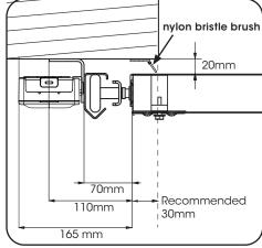
PANELIFT<sup>®</sup> ICON (PFI) with Auto-lock and nylon Bristle Brush measurements for vertical track
