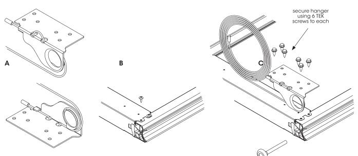
**NOTE:** DO NOT hold cable in place by squeezing the bracket around it as this will cause the cable to fracture and break. Should you need to temporally hold the cable in place during installation before spring tension is applied only secure with sticky tape.
