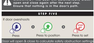
NOTE: If unhappy with the speed or travel limit setting, restart this procedure by resetting the door limit positions as per below first.
