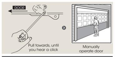
CAUTION: When the opener is manually disengaged, the door is no longer locked. To lock the door manually, re-engage the opener after the door is closed.
