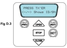
The controller provides several diagnostic tools from within the Diagnostics Menu (Menu 8). This section details the function of each tool and its use.
