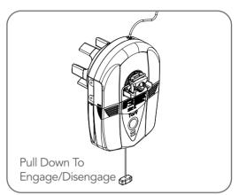
WARNING! Please test the manual release mechanism to ensure that the manual release is easy to operate. No more than 15 kg of force should be required to disengage the door using the manual release cord. If excessive force is required reset the close limit position.
