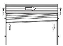
If the door rolls up crooked with the **RIGHT HAND SIDE** higher than the left proceed as follows:
