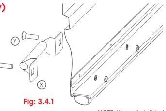
**NOTE:** if handle is fitted the walk through height will be reduced by 80mm.
