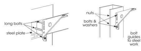
WARNING! Masonary blockwork should be properly filled and reinforced if brackets are to be mounted directly to blockwork with masonry anchors. Where the blockwork is not solidly filled but structurally sound, long bolts should be passed through the blockwork using suitable steel plates under bolt heads. Special consideration should be given to brick type and construction of wall, to ensure satisfactory fixing.
