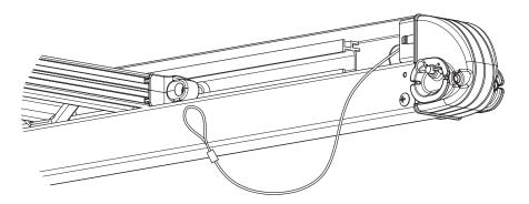
With door in open position disconnect cables & opener if fitted.
