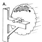
required for satisfactory operation may vary with individual doors depending on size. Final adjustment should be made later.
